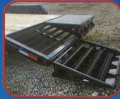
Straight, deck models are available with slide in ramps, stand-up ramps or 2 piece folding beavertail ramps for full width loading.
