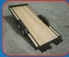
Straight, deck models are available with slide in ramps, stand-up ramps or 2 piece folding beavertail ramps for full width loading.
