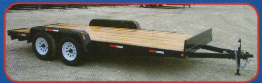
Tilting is hydraulically controlled on full deck tilting models. Available with manual or electric over hydraulic operation.
