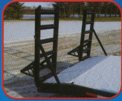
Straight, deck models are available with slide in ramps, stand-up ramps or 2 piece folding beavertail ramps for full width loading.
