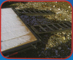
Straight, deck models are available with slide in ramps, stand-up ramps or 2 piece folding beavertail ramps for full width loading.
