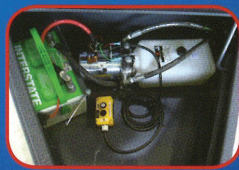
Tilting is hydraulically controlled on full deck tilting models. Available with manual or electric over hydraulic operation.
