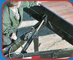
60/40 tilting deck models come with a mechanical lock and a quick shut valve. In addition to cushion the tilt, the valve also allows you to lock the deck in any position.
