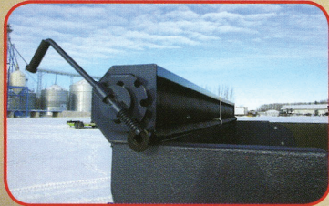
Fold down sides and roll tarps are available. Wall mounted D-Rings are standard.
