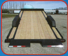
Tilting deck models come with a checkerplate dovetail ramps.
