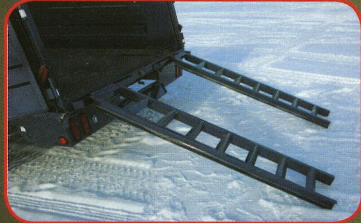
All precision dump trailers come with rear slide-in loading ramps and side step for easy inspection.
