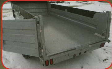
The tailgate can be unlatched from the bottom and set to spread your load or opened from the center out (barn door style). The doors can be latched open for total access and cleanout.
