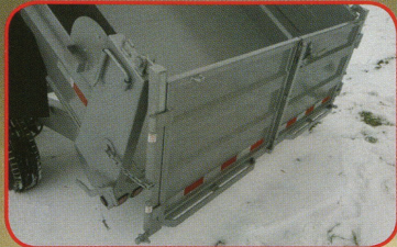
The tailgate can be unlatched from the bottom and set to spread your load or opened from the center out (barn door style). The doors can be latched open for total access and cleanout.
