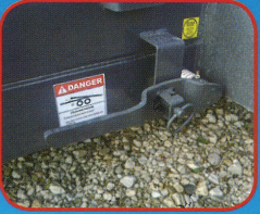
60/40 tilting deck models come with a mechanical lock and a quick shut valve. In addition to cushion the tilt, the valve also allows you to lock the deck in any position.
