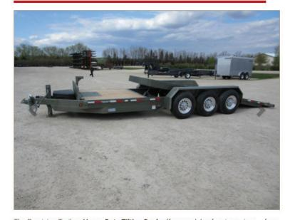
The Precision Trailers **Heavy Duty Tilting Deck** offers models of various sizes – from the partial 60/40, to the full tilting deck running either electric over hydraulic power packs, or a free flowing valve controlled cylinder.
